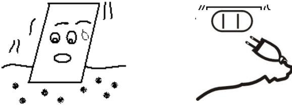
4. For a better dehumidifying effect, the areas to the front, rear and above the unit should be clear and free from any obstacles which will block the air flow of the unit. Do not block any air inlet or outlet grilles – keep clear of hanging drapes, curtains and furnishings – **DO NOT COVER, as specified under safety information section a clearance of 50cm should be maintained all around the appliance when it is in use.**
