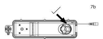
Ensure that the cable does not obstruct the Transducer Disc. To prevent the cable becoming pinched between the nozzle and the sump, place the cable in the slot in the wall of the sump.
