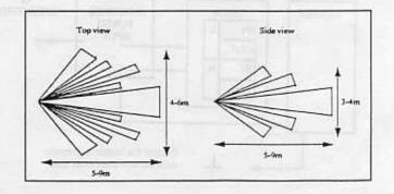
The control must be mounted in a location that allows the PIR detector good unobscured coverage of the room occupants (see detector pattern above). Normally mounting at wall switch height is desirable.
