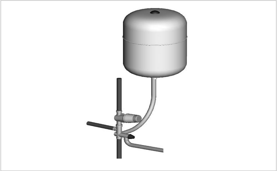
Figure 10 – Installation expansion vessel (optional for standard SCxn d/i cylinders, mandatory for solar SCxn d/I cylinders)
