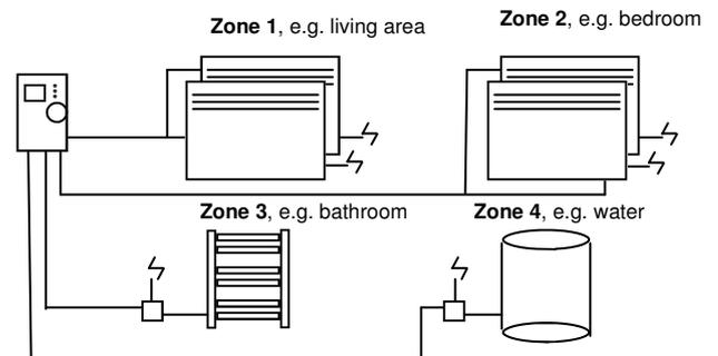
The RXPW4 controller allows control of multiple Dimplex heaters from a single point.
