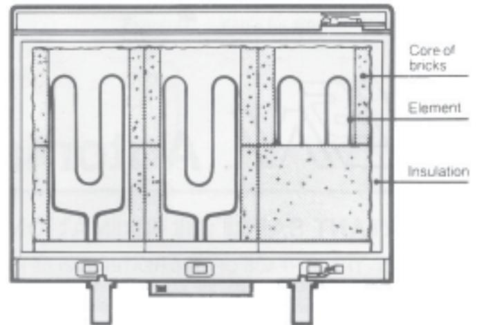
In the morning, when the core is at its hottest, the amount of heat being transmitted through the insulation and emitted as radiant heat is at its greatest and the heater feels hot over most of its upper outer surfaces. *Diagram 2.*
