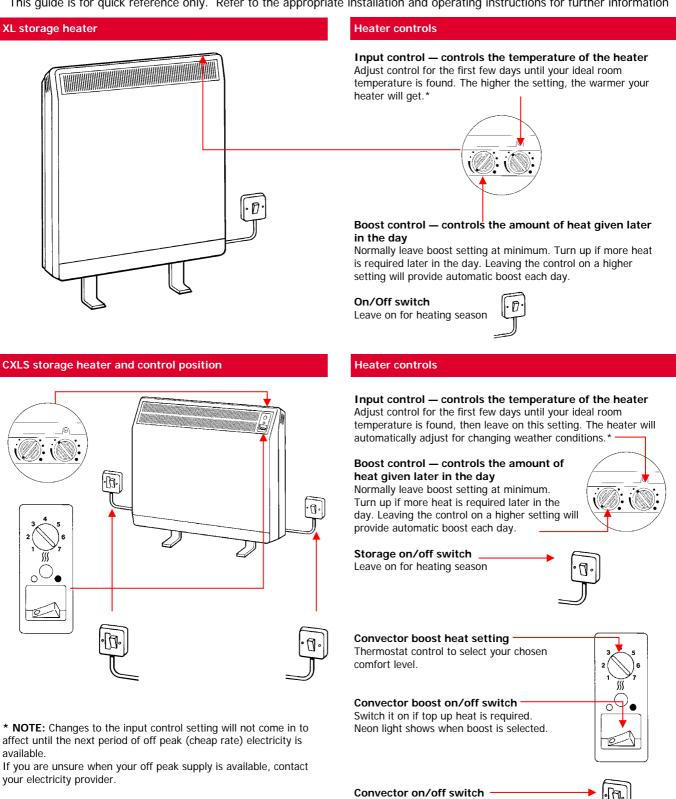
WARNING: Walls, curtains and furniture should be at least 75mm away from the top and sides of the heater. Furniture and other obstructions should be at least 150mm from the front of the heater. DO NOT COVER or obstruct the air inlet or outlet grilles. PLEASE REFER TO THE OPERATING AND INSTALLATION INSTRUCTIONS FOR FURTHER SAFETY ADVICE.
