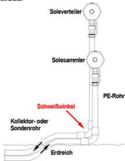
Fig. 3.7: Installation of the pipelines with welding on the brine distributor
