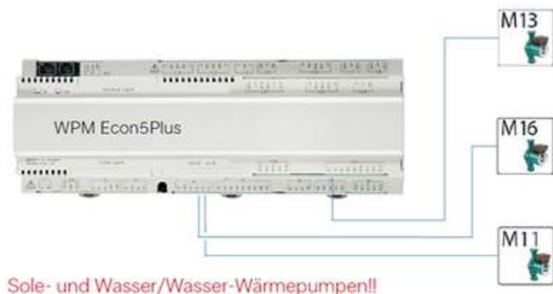
Fig. 7.49: Electrical wiring of control signal 0 - 10V and PWM for brine / water heat pumps on the WPM Econ5Plus
