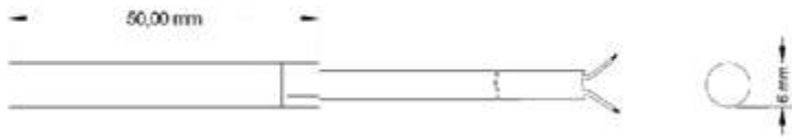
Fig. 7.4: Dimensions of the NTC 10 heating sensor with metal sleeve
