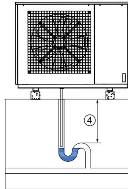
Fig. 6.8: Condensate pipe in channel over siphon
