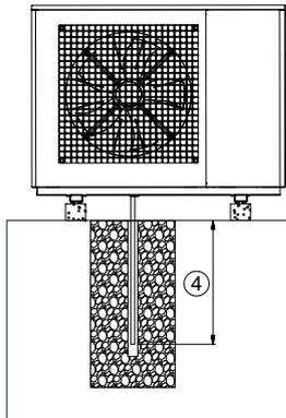
Fig. 6.7: Condensate drain in gravel
