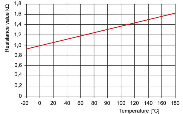
Fig. 7.10:Sensor characteristic curve PT 1000
