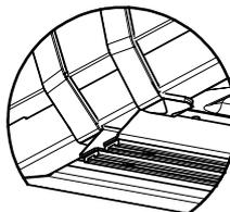
After transportation, the transport fastening in the device is to be removed from both sides of the base.
