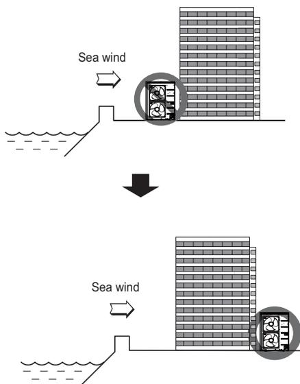
Case 2: If the outdoor unit is installed in the direction of the sea wind, set up a wind guard to catch the sea wind.
