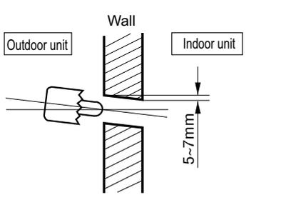
For the safe drainage of the condensate, the condensate drain must be positioned in such a way that no frost build-up can occur. The frost line can vary according to the climatic region. The regulations of the countries in question must be observed.
